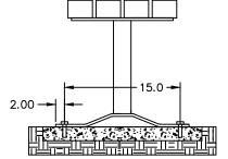
FRAMES SHOULD BE ANCHORED TO A CONCRETE PAD PROVIDED BY THE CUSTOMER
