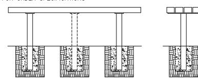
INGROUND MOUNT FRAMES SHOULD BE BURIED IN A SUFFICIENT AMOUNT OF CONCRETE TO SECURELY HOLD UNIT IN PLACE FOR INTENDED USE AND ENVIRONMENTAL CONDITIONS
